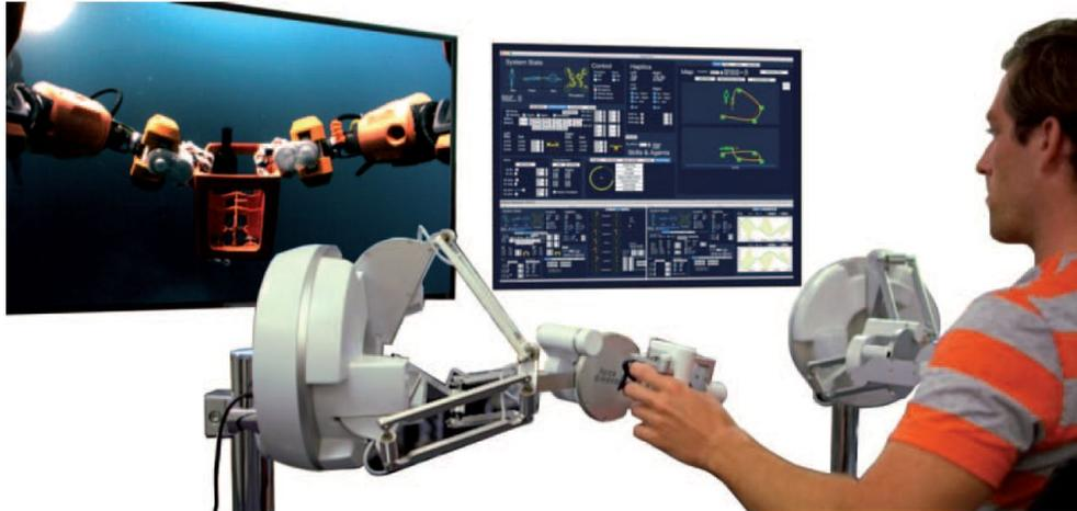
Figure 3: A human operator guiding the robot in an underwater bimanual task through the haptic-visual interface (Khatib et al., 2016)
