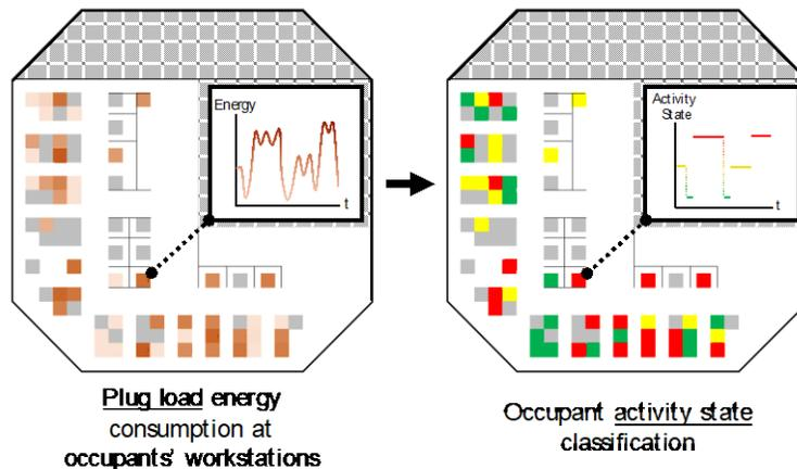
Figure 2: Inferring occupant activity states from plug load sensor data.
