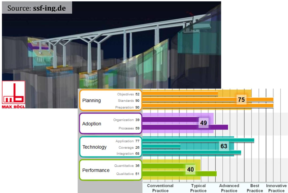
Figure 2: VDC Scorecard Assessment of Filstal Bridge
