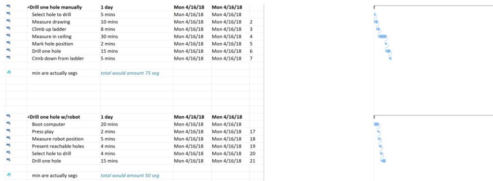
Fig. 3: Schedule drill one hole manually and with robot
